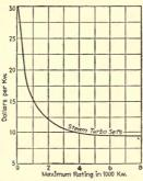
Fig. 273.—Approximate relative costs of turbo-generator units. (Cost of labor and materials are now fluctuating so widely that it is not feasible to give actual costs.)
